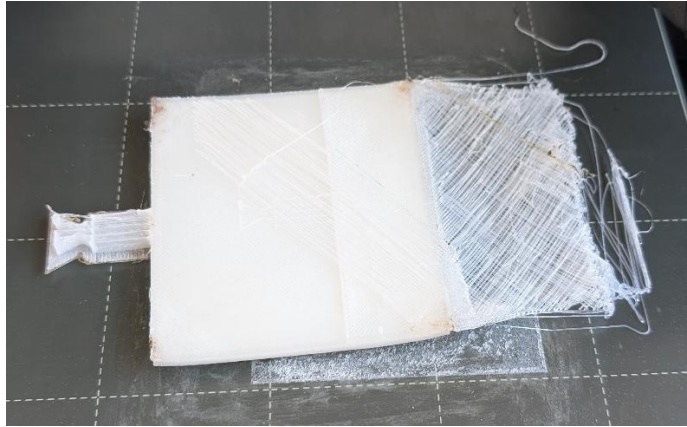
Figure A – Warping and burning of reservoir holder surface using Nylon filament (a), Shifting of model during 3D printing as a result of not adhering to the printer bed (b)
