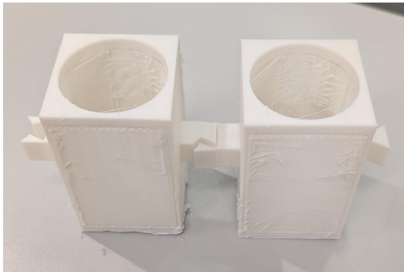
Figure D – Resolution of 3D printer preventing dovetail from fitting, support structure of wall too dense, many strands of filament remaining after print.
